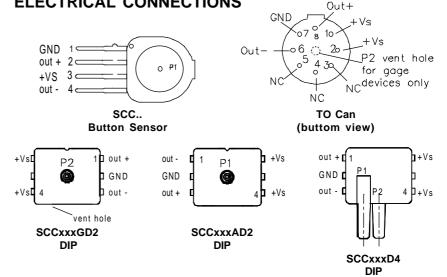
The polarity indicated is for pressure applied to
